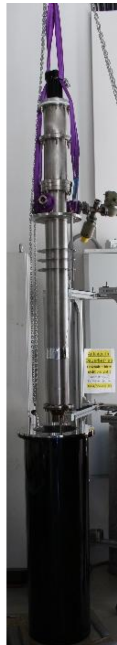
Cryo-Tribometer in shroud and section view
