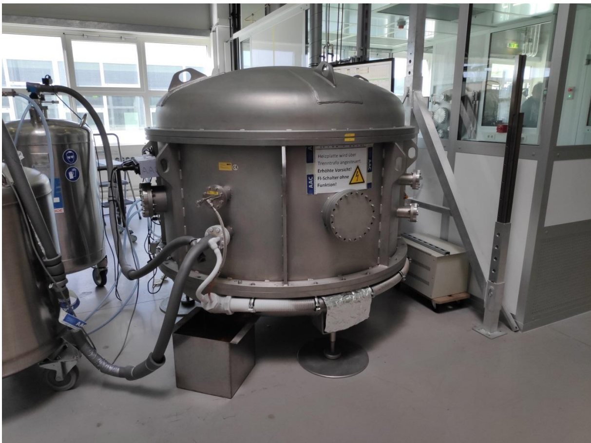
Figure 1: Overview of LVC Thermal Vacuum Chamber
